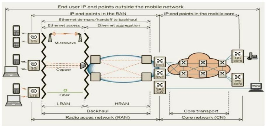
• LRAN (access RAN) includes multiple physical technologies (uwave, copper, fiber etc)
